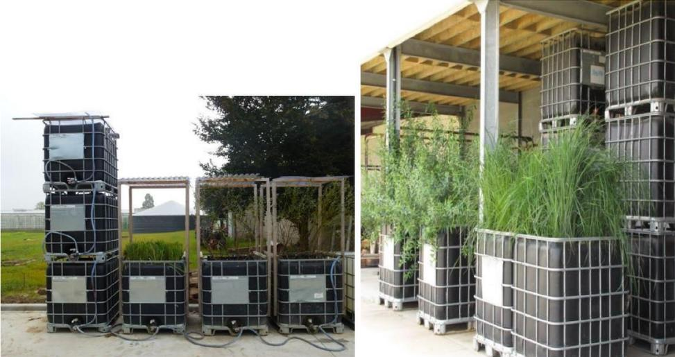
**Figure 23: Biofilters in practice. Photo: PCfruit test centre, Sint-Truiden.**
