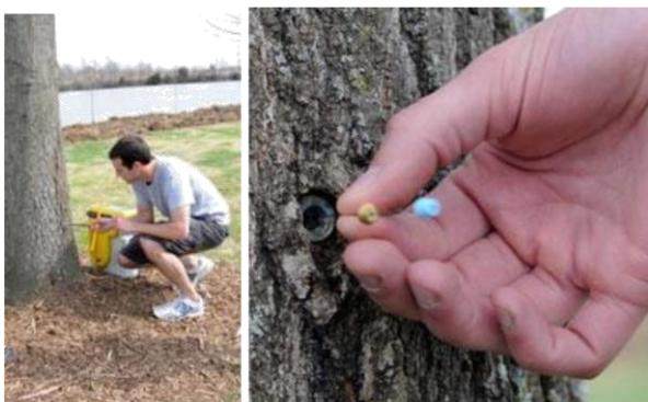
**Figure 25: Drilling down to sap flow and SPME or SPS sampling. Source: Joel Burken lab, Missouri S&T, USA.**
