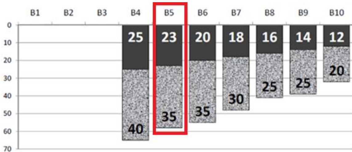
Figure 5: Recommended road structure for bituminous roads in relation to the different traffic classes (following AWV [50]) 4 .
