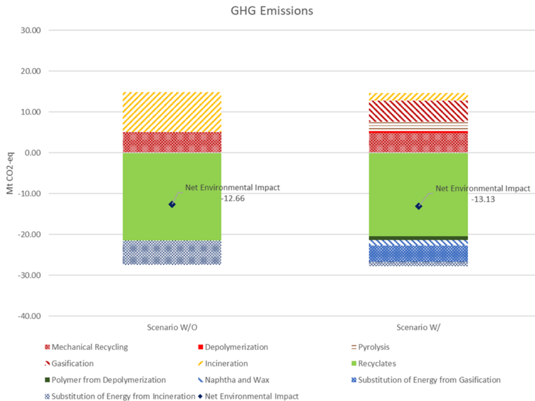
Figure 15: Results of GHG emissions, expressed as Mt CO 2 -eq, of the two scenarios (Scenario W/ and Scenario W/O) in 2030. Notice that values above the zero line are burdens, while values below the zero lines are savings.
