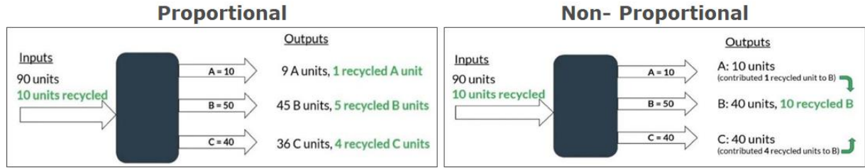
Figure 8: Illustration of the proportional and non-proportional allocation method in a one-step recycling process. In the proportional method, the allocation is applied to each output to guarantee an actual physical and chemical relationship of the recycled material or product with the waste feedstock. In the non-proportional, the allocation is applied entirely to one single output. The choice of what kind of allocation is used, is out of the scope of this report and is up to the operator. What matters for the calculation of the recycling yield is the total amount of recycled material (sum of individual recycled materials).
